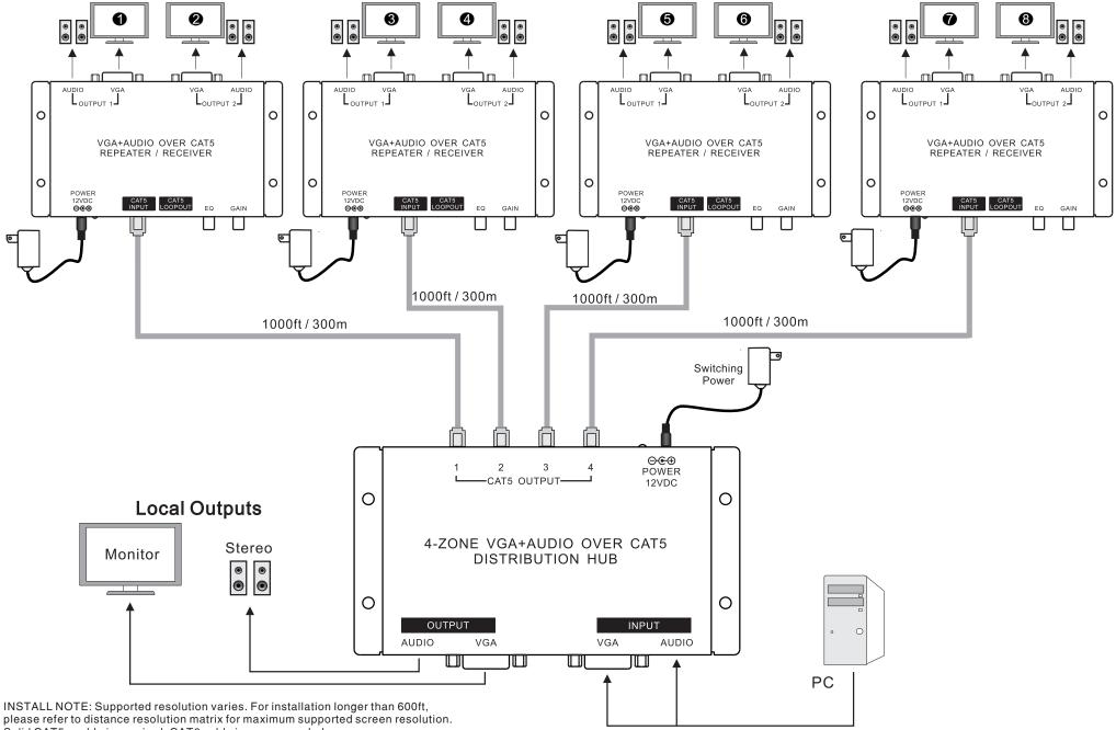
Solid CAT5e cable is required, CAT6 cable is recommended.
