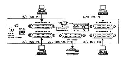
Fig. 2-1-1 AS-411P's 4 IN/1 OUT Configuration
