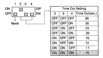
Fig 2-2-3 AS-411S/811S Auto Switch's DIP Switch Setting
