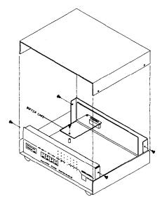
Fig 2-3-I The AS-41 | P's Buffer Card Installation
