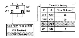
Fig 2-2-1 AS-411P Auto Switch's DIP Switch Setting
