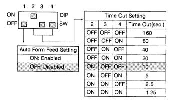
Fig 2-2-2 AS-811P Auto Switch's DIP Switch Setting
