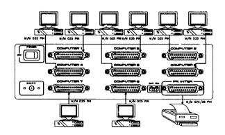
Fig. 2-1-2 AS-811P's 8 IN/1 OUT Configuration
