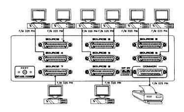
Fig. 2-1-4 AS-811S's 8 IN/1 OUT Configuration
