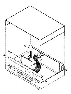
Fig 2-3-2 The AS-81 1 P's Buffer Card Installation
