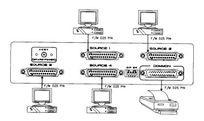
Fig. 2-1-3 AS-411S's 4 IN/1 OUT Configuration
