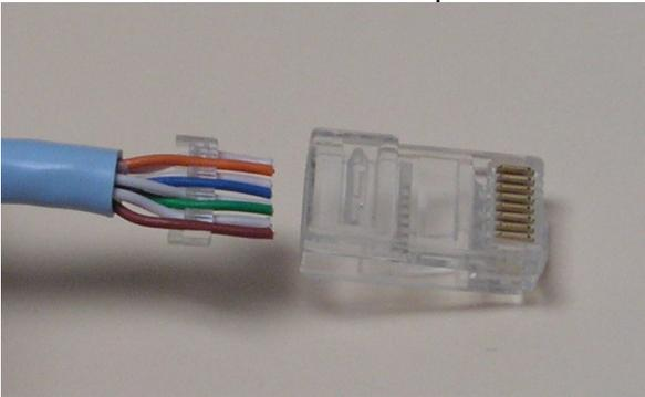
8. Insert wires in to connector and crimp
