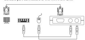
2. Use the extender cables (as described in the Hardware Requirements section), to connect the monitor, keyboard and mouse ports of the PCs to the MiniView CPU Ports, as shown in the diagram below.
