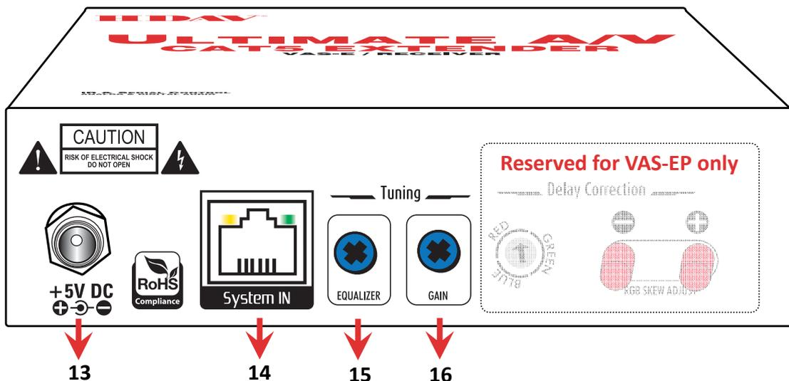
13. **+5V DC** power jack: connect to 5V DC power supply unit
