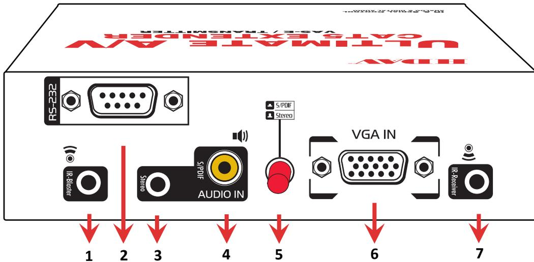
1. **IR-Blaster:** connect to IR blaster for IR pass-thru from RX to TX
